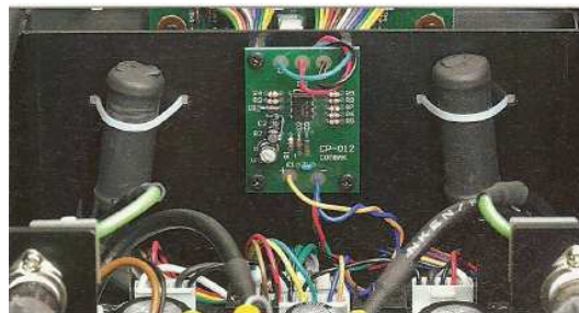
The black Enacom filters are used only to eliminate front LED interference
