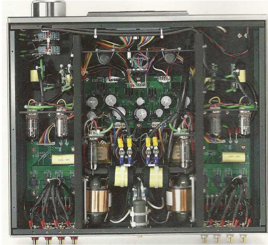
Double mono: the insides of the CAT-777 MKII are designed symmetrically right down to the length of the cables
