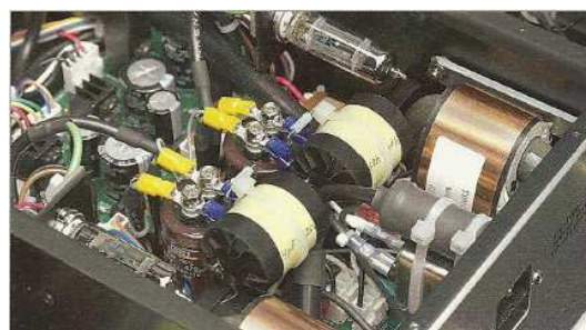
Hand-wound film capacitor (black jacket, yellow wrapper)
